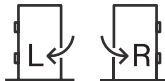
When ordering, select left (L) or right (R) hinge as seen from outside.
